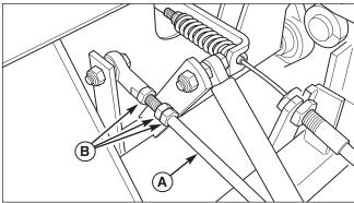
Figure 31. Neutral Adjustment (RH side shown)
